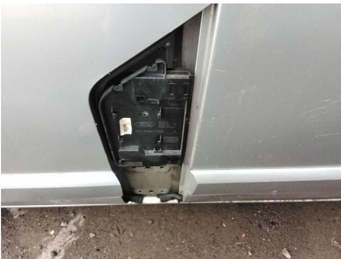
7: Door Moulding nsf Missing Replace
