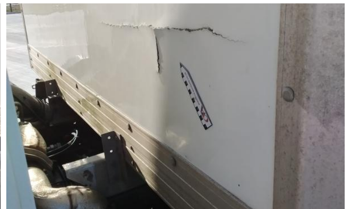
6: A Post ns Scratched Over 25mm Thru Paint
