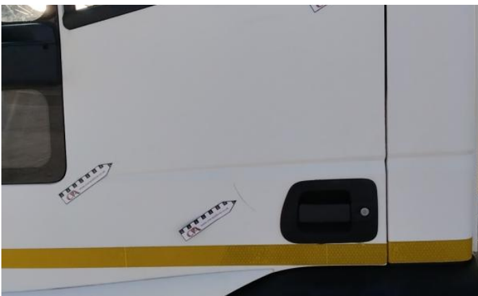
5: Wing nsf Scratched Over 25mm Thru Paint
