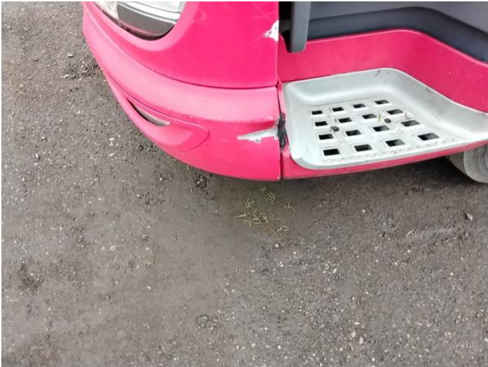
3: Bumper Front Dented Over 30mm
