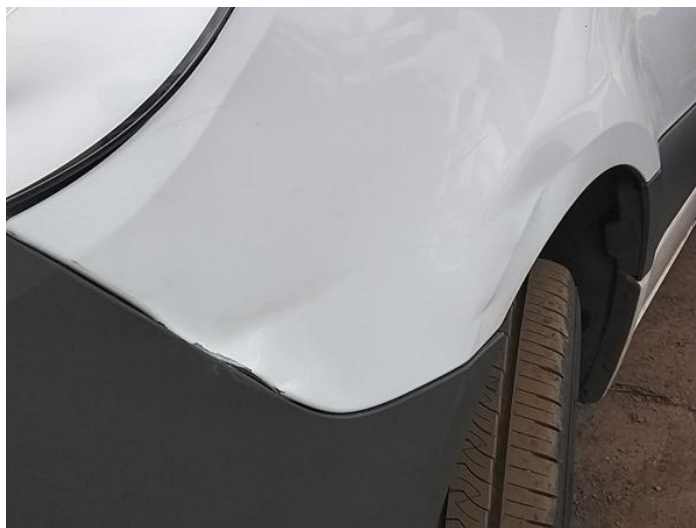
2: Wing osf Dented With Paint Damage
