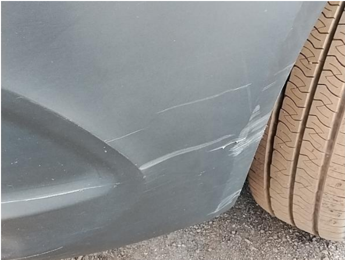
3: Bumper Front Moulding Scuffed (Unpainted) Over 100mm
