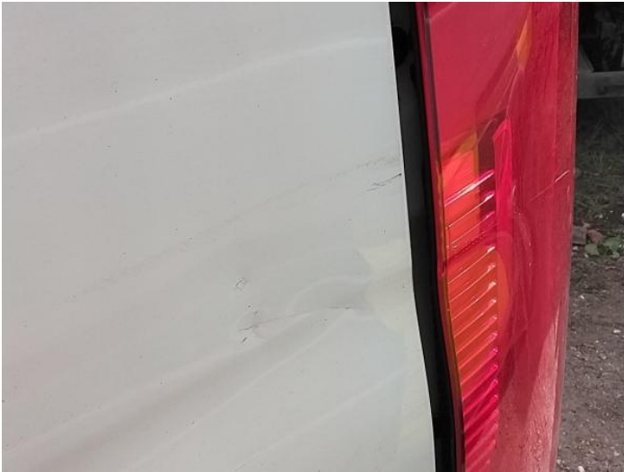
9: Panel Rear Dented Between 10mm + 30mm
