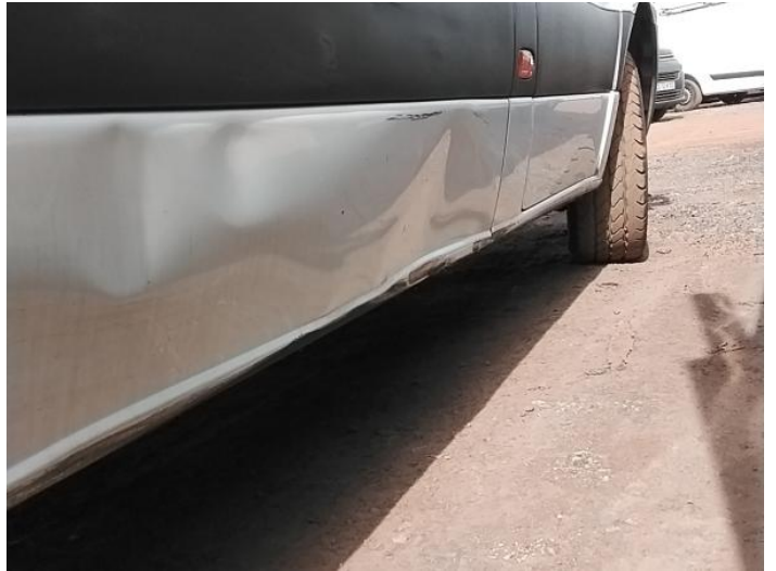
16: Sill ns Dented Over 30% Of Panel
