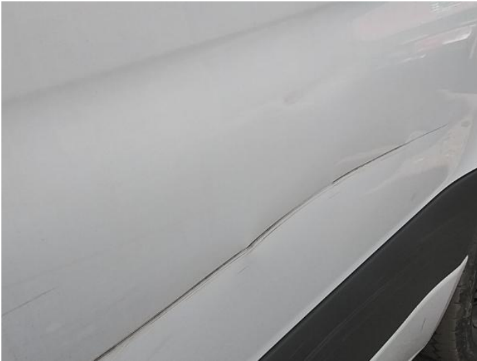
15: Panel Rear Scratched Over 25mm Thru Paint
