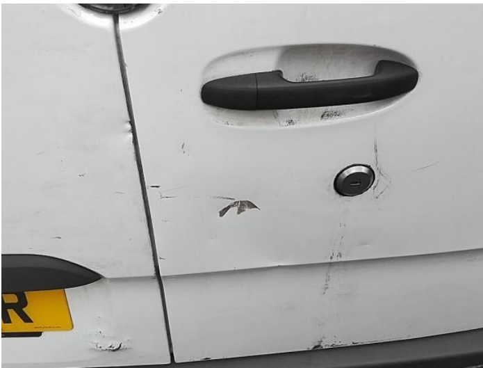
11: Door nsr Scratched Over 25mm Thru Paint
