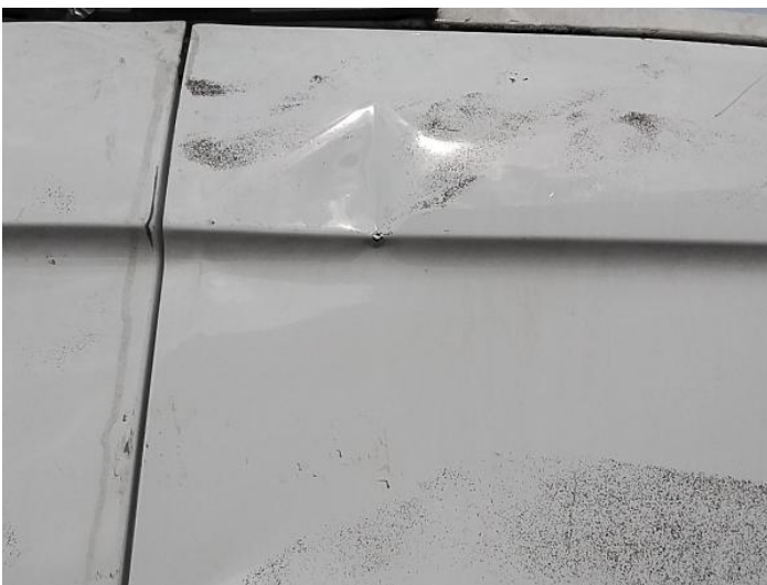
13: Door nsr Dented Over 30mm
