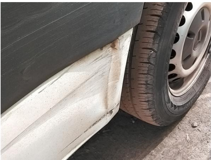
7: Sill os Dented With Paint Damage
