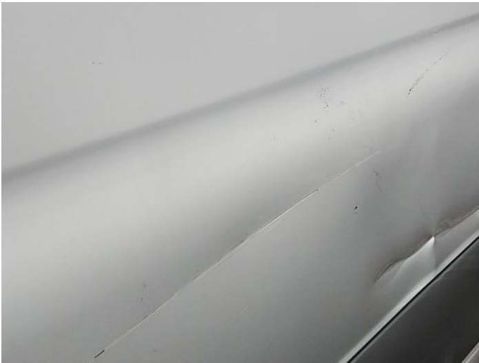
17: Panel Front Scratched Over 25mm Not Thru Paint
