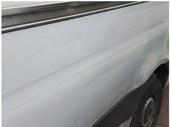
6: Panel Rear Scratched Over 25mm Thru Paint
