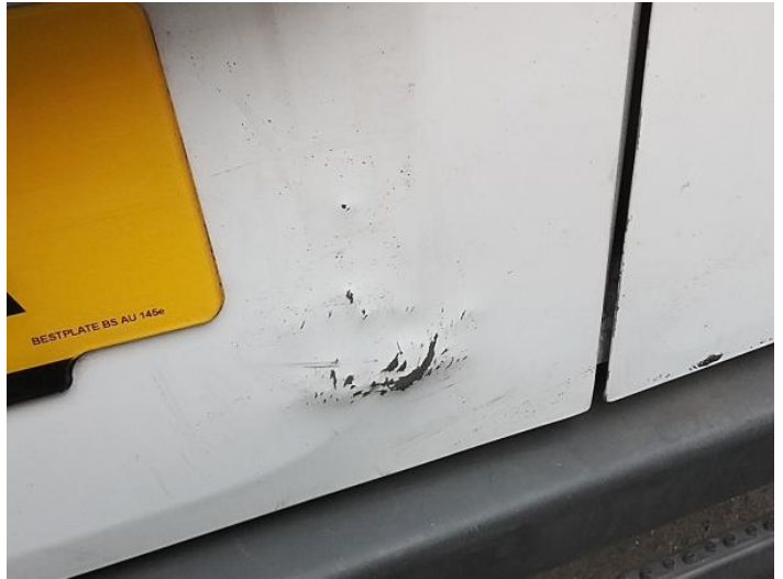
10: Door osr Dented With Paint Damage
