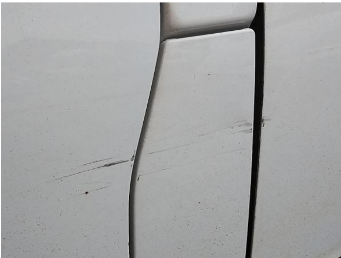
5: Door osf Scratched Over 25mm Thru Paint
