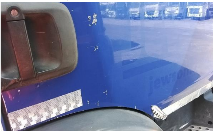
5: Door nsf Dented With Paint Damage
