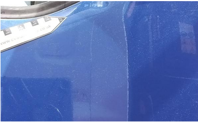
3: Bumper Front Scratched Over 100mm Thru Paint
