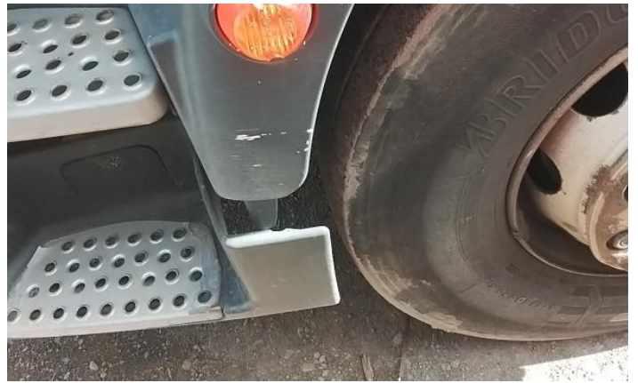
4: Bumper Front Scratched Over 100mm Thru Paint
