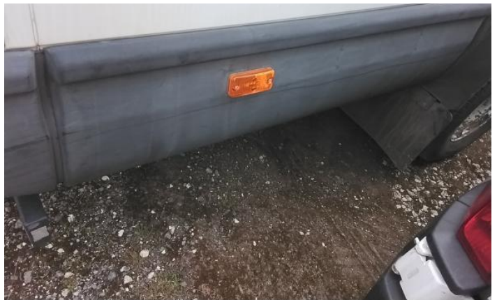
6: Qtr Panel nsr Dented Over 30mm
