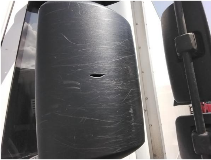
3: Door Mirror Assy osf Broken Replace
