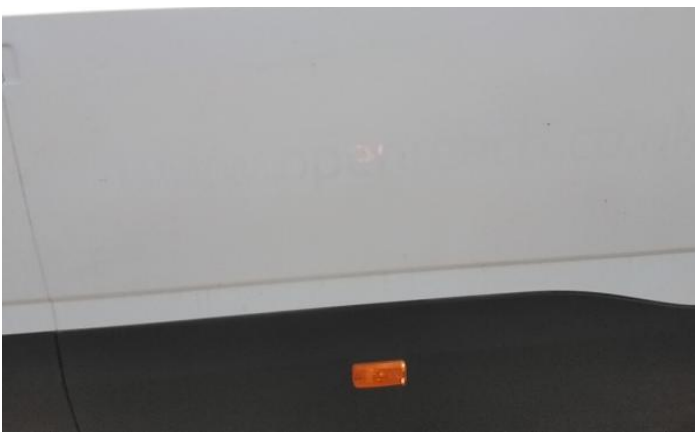
5: Door osr Dented Over 30mm
