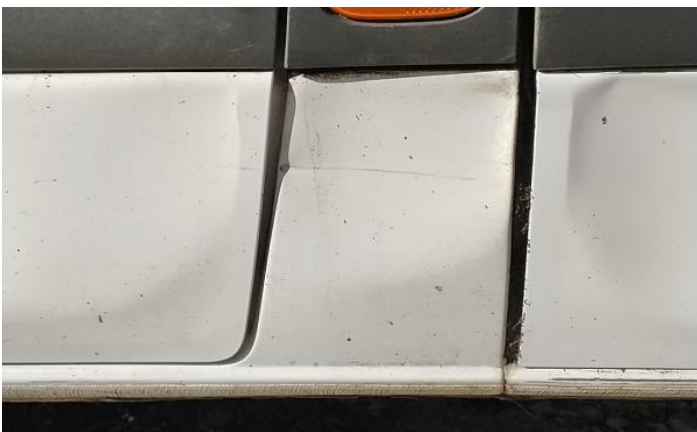
11: Door nsf Scratched Over 25mm Not Thru Paint
