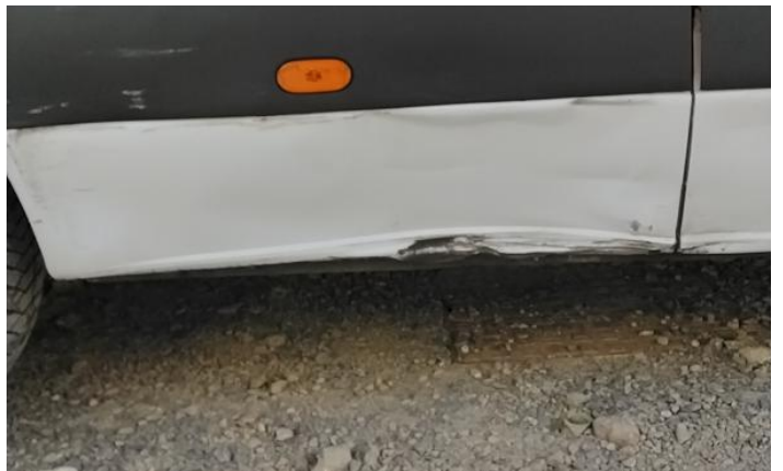
24: Qtr Panel osr Dented Over 30mm
