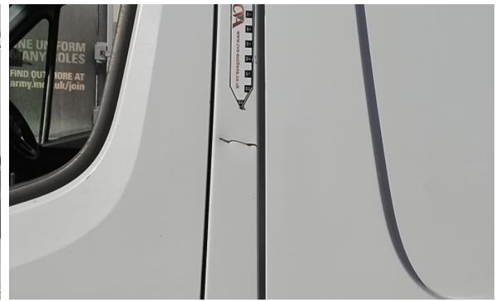
10: Door Moulding nsf Scuffed (Unpainted) Over 100mm
