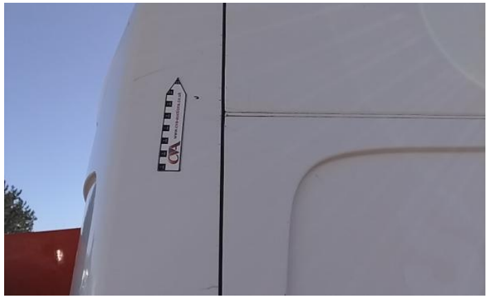
22: Door osr Dented Over 30mm
