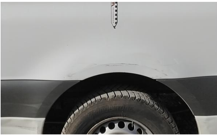
15: Door Moulding nsr Scuffed (Unpainted) Over 100mm
