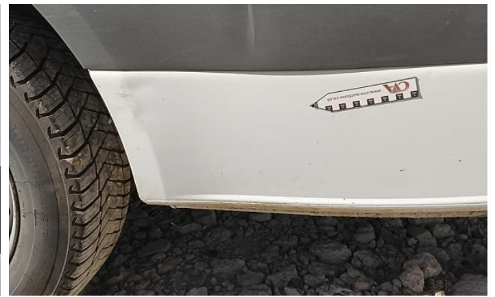
16: Qtr Panel nsr Dented With Paint Damage
