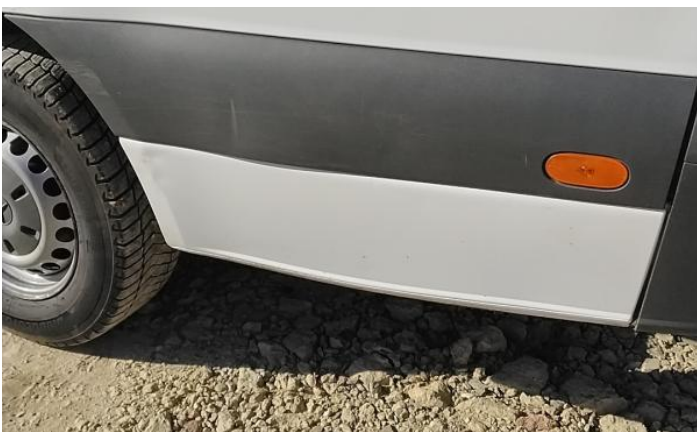
17: Qtr Panel nsr Scratched Over 25mm Not Thru Paint
