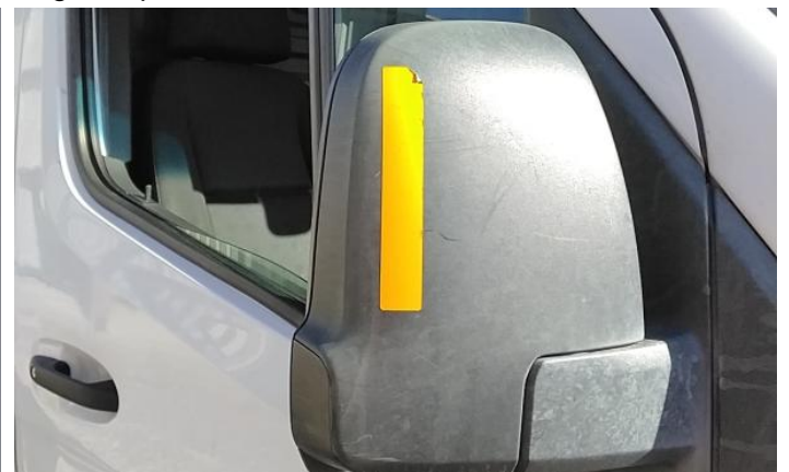
30: Door osf Chipped Edge Chip
