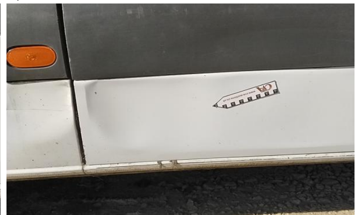
12: B Post ns Scratched Up To 25mm Thru Paint
