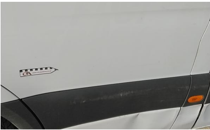
9: Door nsf Dented With Paint Damage
