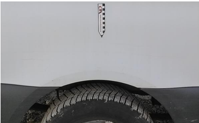
23: Bumper Rear Moulding Scuffed (Unpainted) Over 100mm
