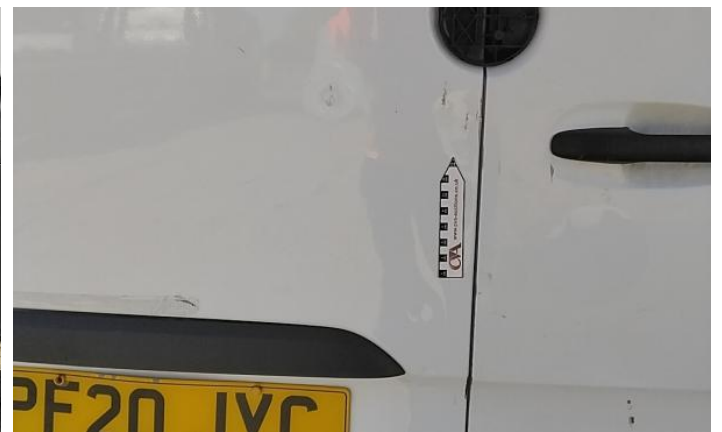
18: Qtr Panel nsr Dented Between 10mm + 30mm
