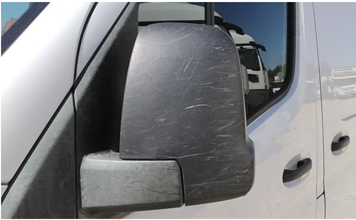
3: Wing nsf Scratched Over 25mm Not Thru Paint
