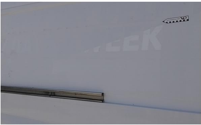
9: Door nsr Dented Over 30mm
