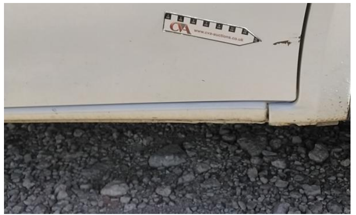
16: Qtr Panel osr Dented With Paint Damage
