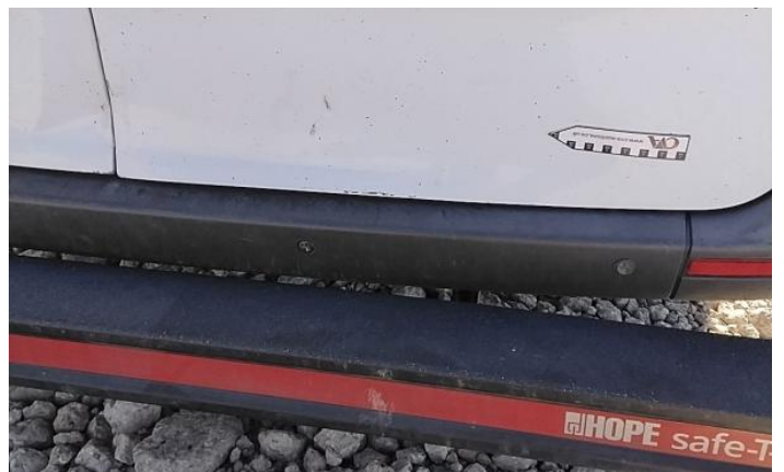
12: Door nsr Dented Over 30mm
