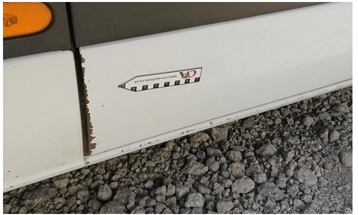
4: Wing nsr Scratched Up To 25mm Thru Paint
