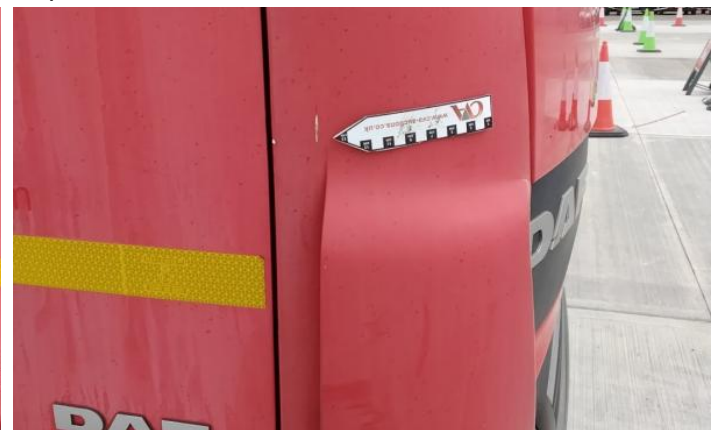
6: Qtr Panel osr Cracked Replace
