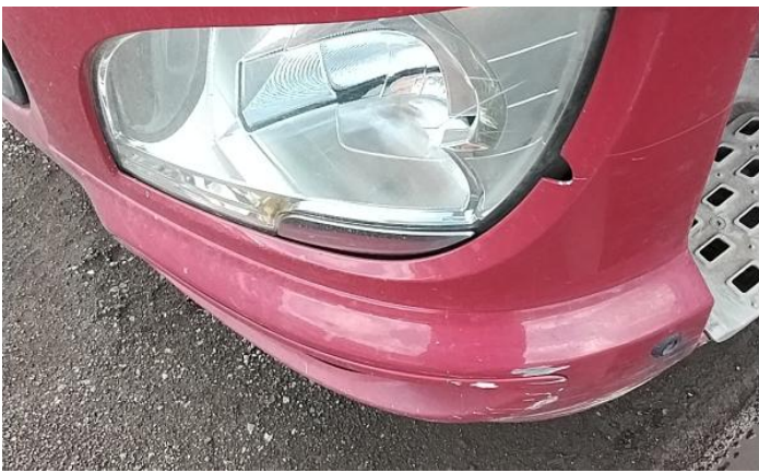
3: Bumper Front Scratched Over 100mm Thru Paint
