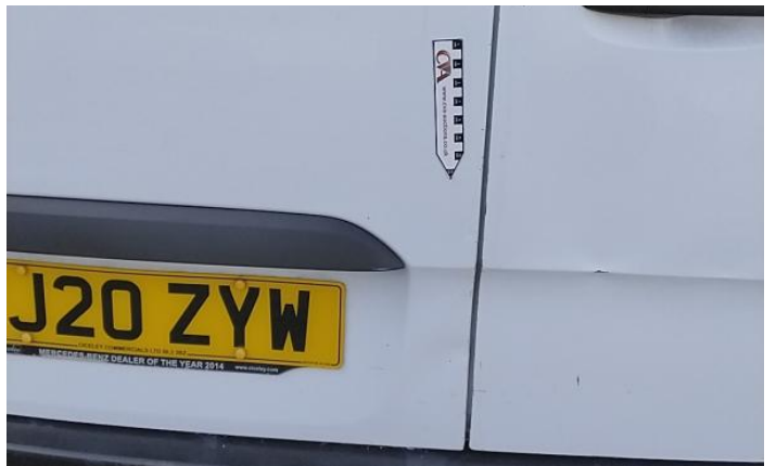
18: Door osr Dented Between 10mm + 30mm
