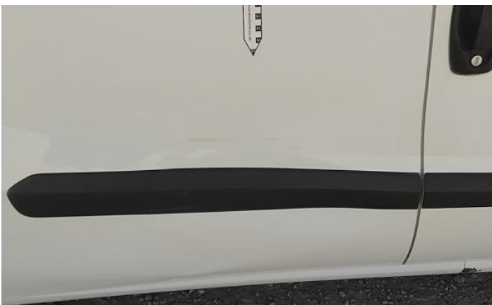
5: Door nsr Dented Between 10mm + 30mm
