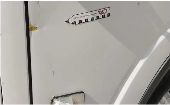
3: Bonnet Chipped Multiple Chips
