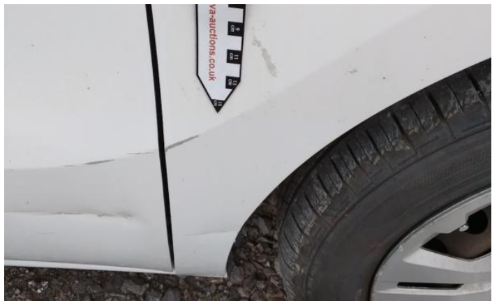
16: Door osf Dented With Paint Damage
