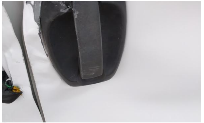
10: Door nsf Dented Hail - Severe
