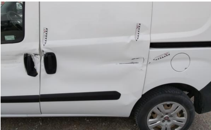
11: Handle Outer nsf Broken Replace
