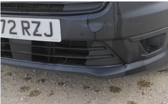
3: Panel Front Scratched UpTo 25mm Thru Paint
