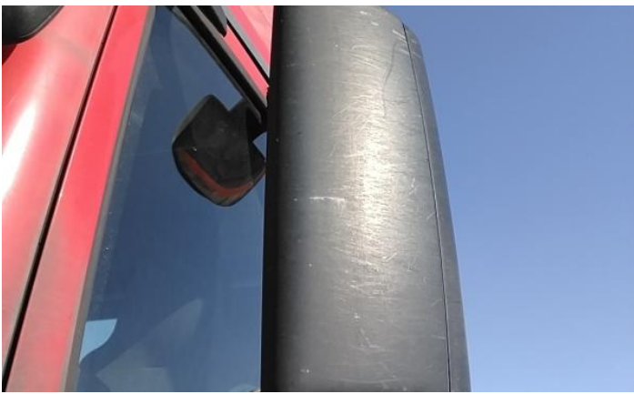
3: Bumper Front Moulding Scuffed (Unpainted) Over 100mm
