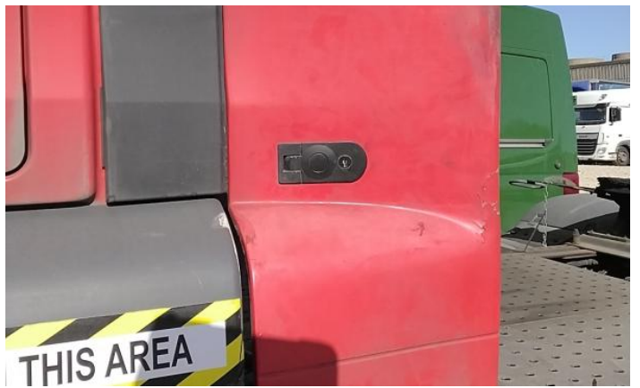
4: Wing nsf Scratched Over 25mm Thru Paint
