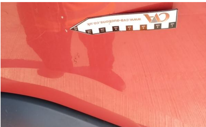
11: Door osf Scratched Over 25mm Thru Paint
