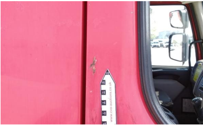
9: Door nsf Scratched UpTo 25mm Not Thru Paint
