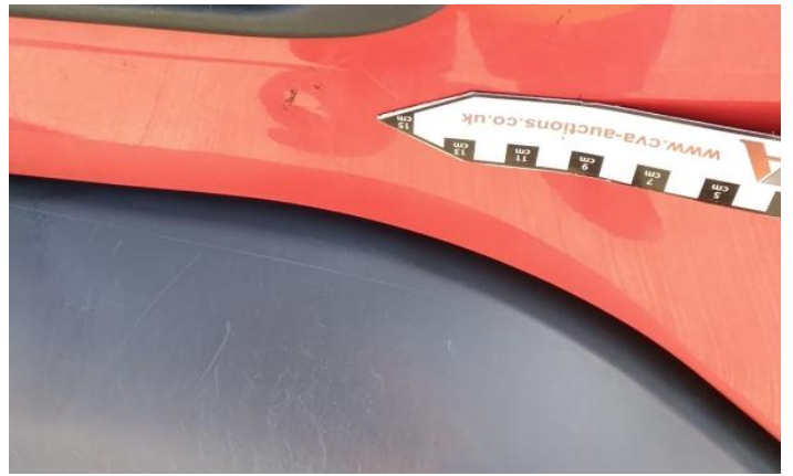
10: Door nsf Dented With Paint Damage
