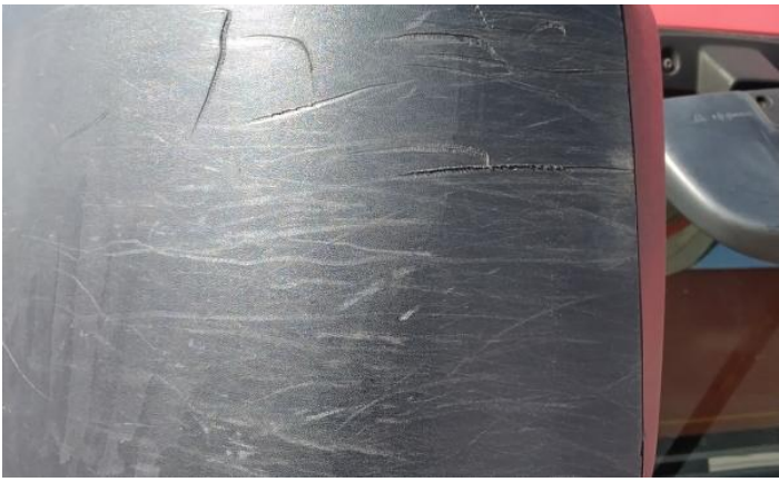
15: Door osf Scratched Over 25mm Thru Paint
