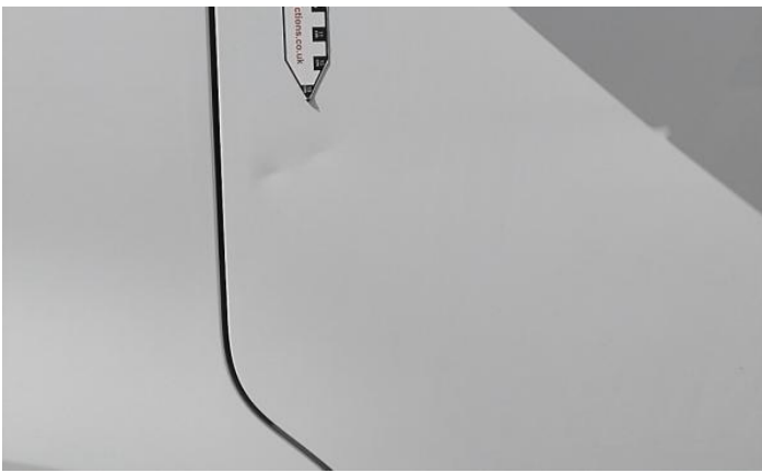
9: Fuel Flap Dented Between 10mm + 30mm
