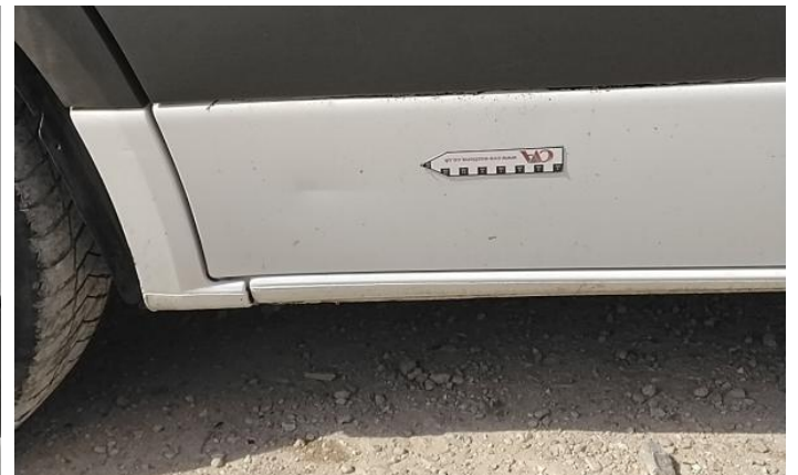
6: Bumper Front Moulding Scuffed (Unpainted) Over 100mm
