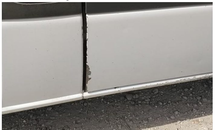
12: Door nsr Dented With Paint Damage
