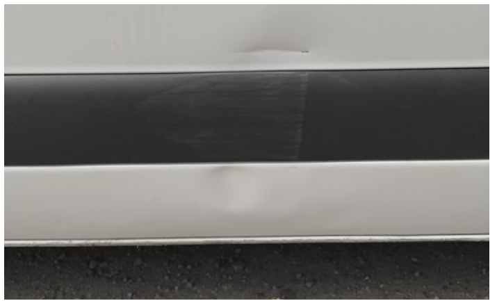
10: Door nsf Dented Between 10mm + 30mm
