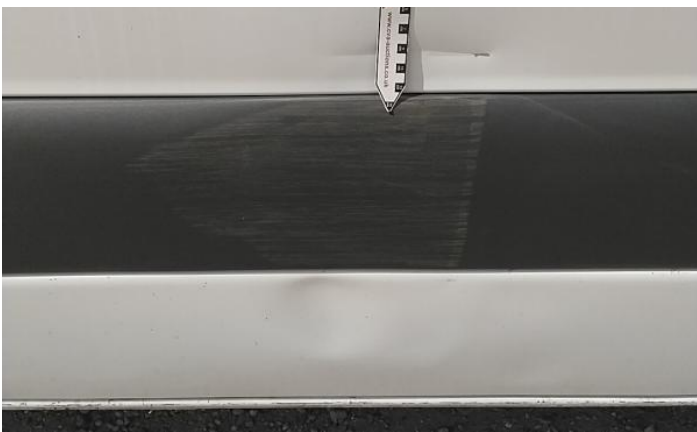
11: Door nsf Dented Between 10mm + 30mm
