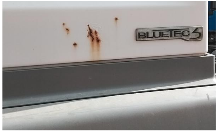
4: Door nsf Chipped Multiple Chips
