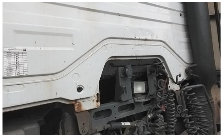
6: Qtr Panel nsr Rusted Over 5mm
