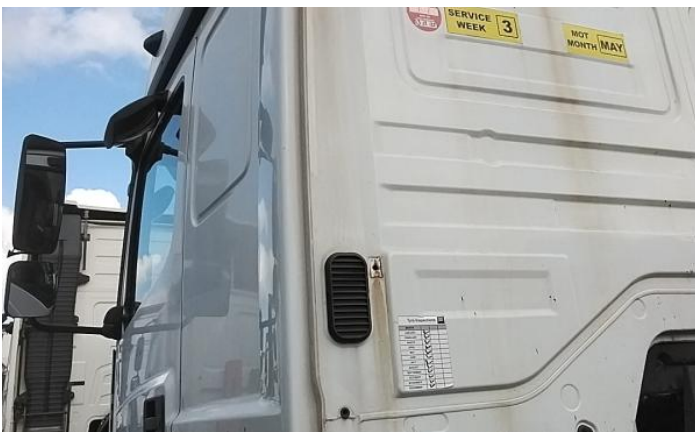
5: Wing nsf Scratched Over 25mm Thru Paint
