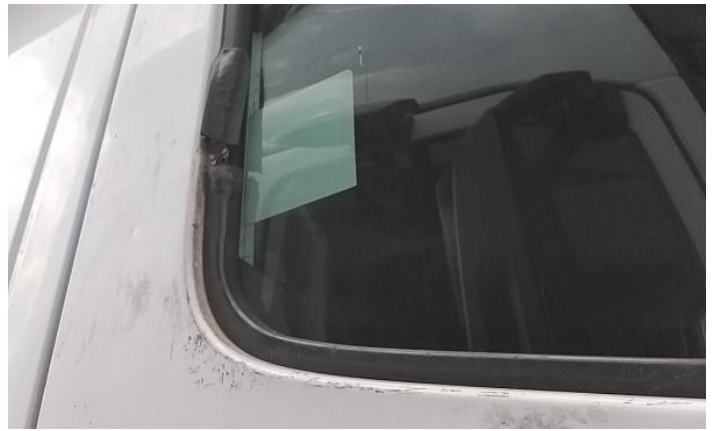
10: Door osf Dented With Paint Damage
