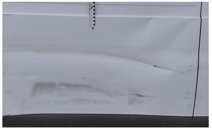
28: Qtr Panel osr Dented With Paint Damage
