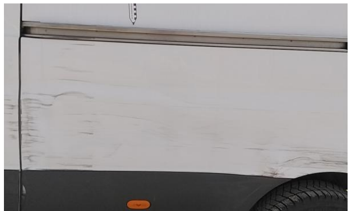
12: Door nsr Dented Over 30mm
