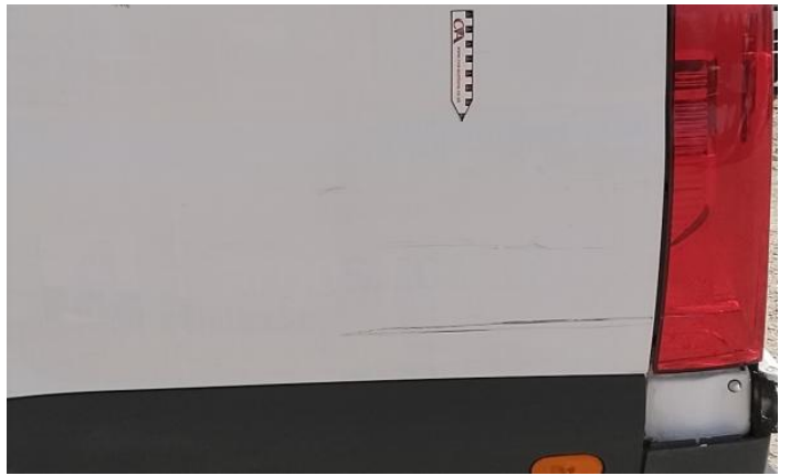
16: Qtr Panel nsr Dented With Paint Damage
