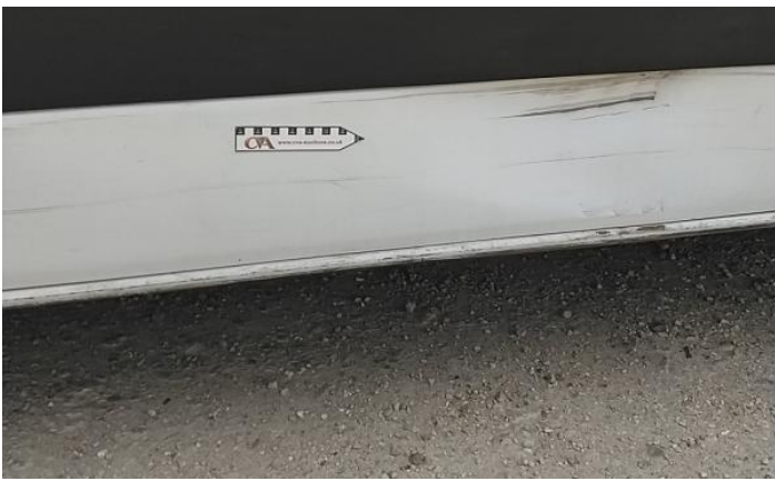
9: Door nsf Dented Over 30mm
