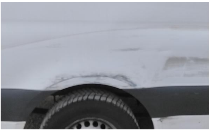
27: Qtr Panel osr Scratched Over 25mm Not Thru Paint
