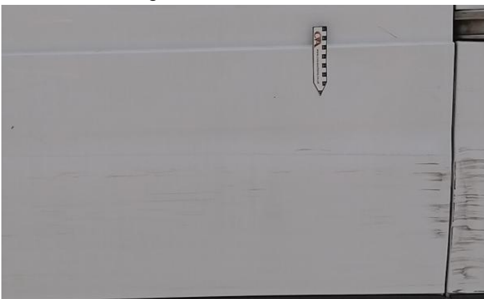
11: Door nsr Dented With Paint Damage
