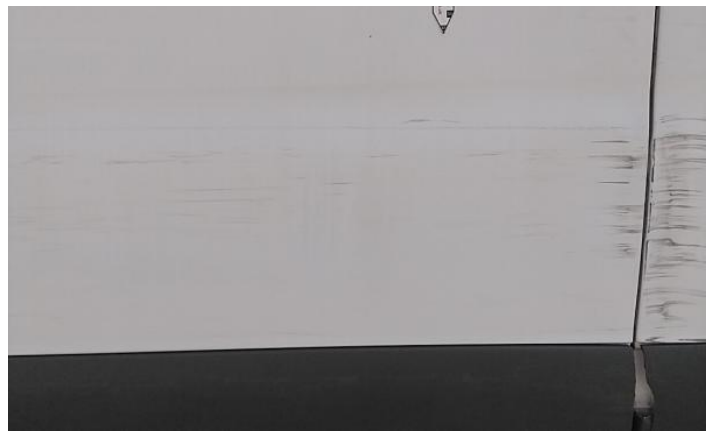
10: B Post ns Dented With Paint Damage
