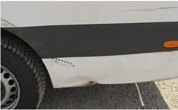
15: Sill ns Dented With Paint Damage
