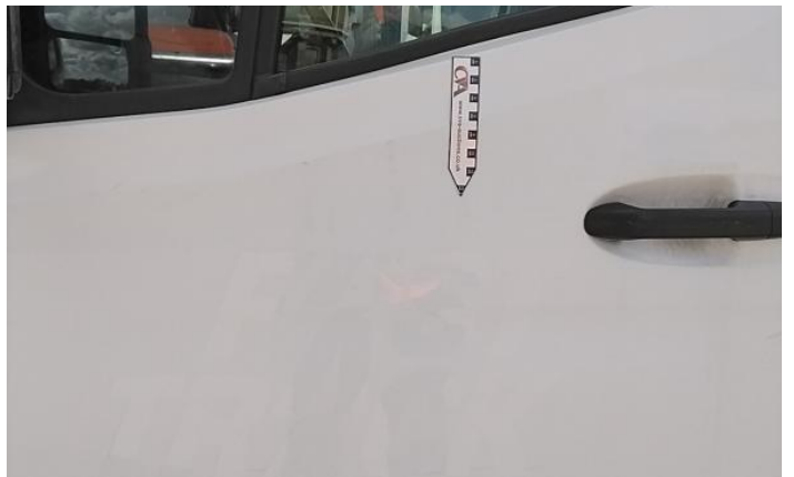
6: Wing nsf Dented With Paint Damage
