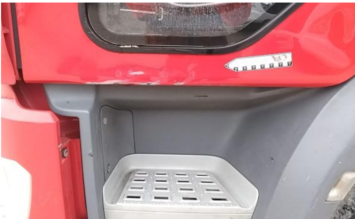
5: Wing nsf Cracked Replace
