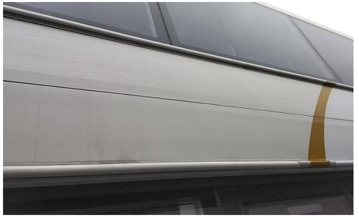
4: A Post ns Scratched Over 25mm Thru Paint
