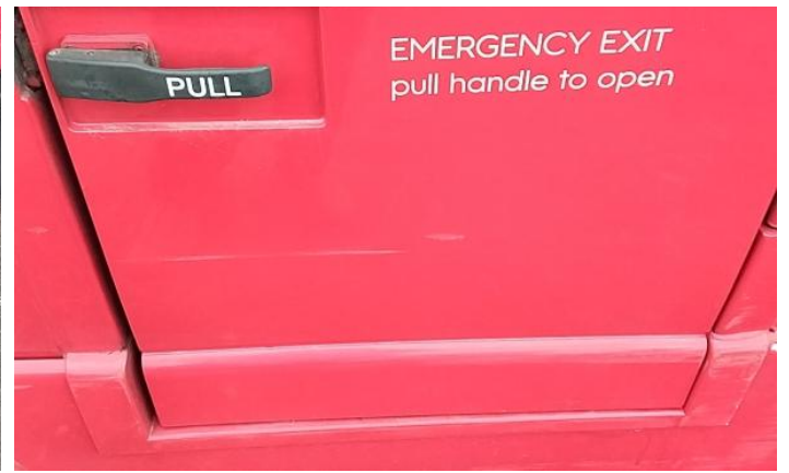
16: Qtr Panel Moulding os Scratched (Painted) Over 25mm Thru Paint
