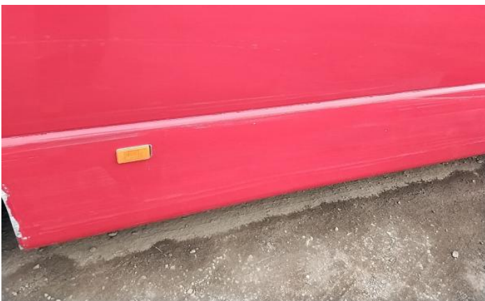
17: Qtr Panel Moulding os Scratched (Painted) Over 25mm Thru Paint
