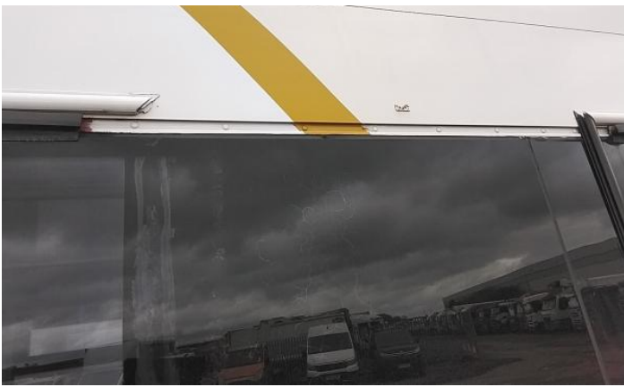
21: Qtr Panel Moulding os Scratched (Painted) Over 25mm Thru Paint
