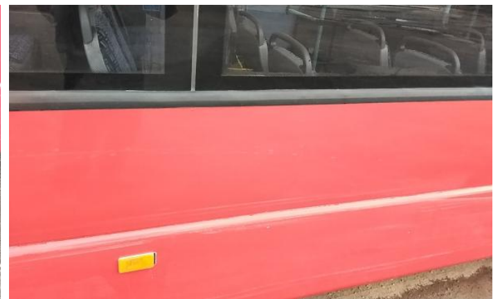
18: Door osr Scratched Over 25mm Thru Paint
