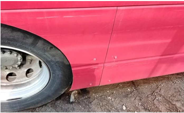
9: Qtr Panel osr Dented Over 30mm
