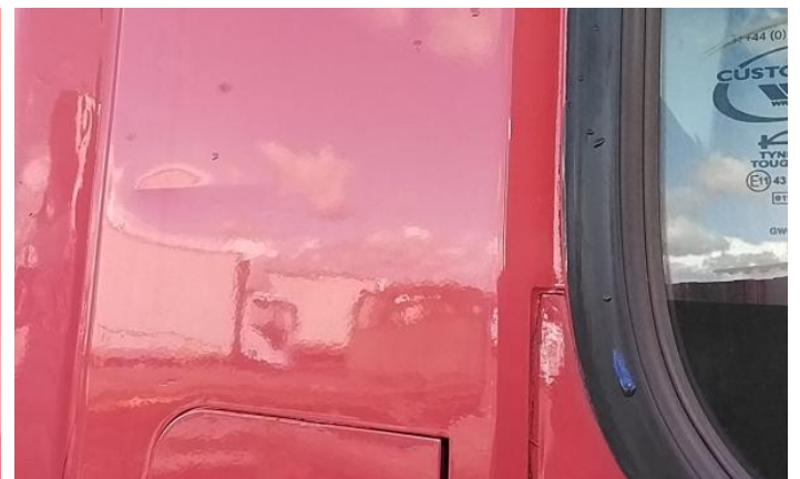
6: Qtr Panel nsr Dented Over 30mm
