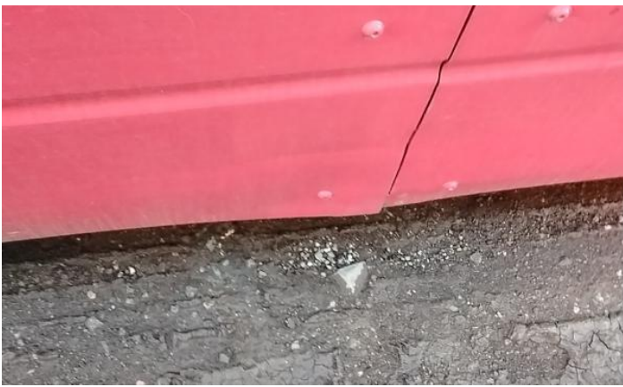
3: Bumper Front Moulding Scratched (Painted) Over 25mm Thru Paint
