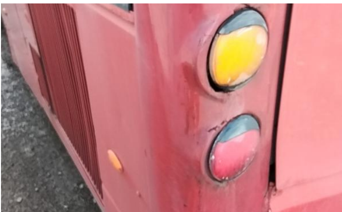
5: Qtr Panel nsr Dented Over 30mm
