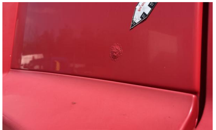
6: Bumper Front Rusted Over 5mm
