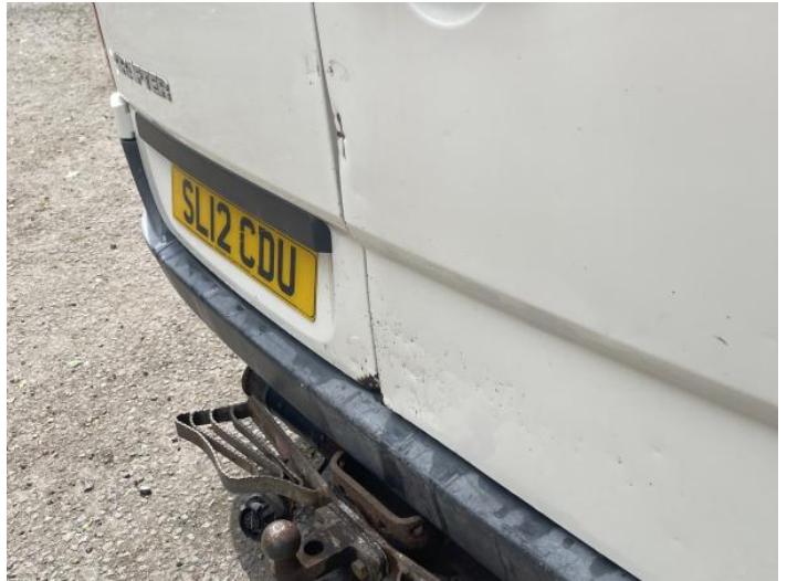
10: Tailgate Dented Over 30mm
