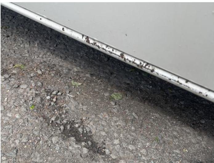
13: Sill ns Rusted Over 5mm
