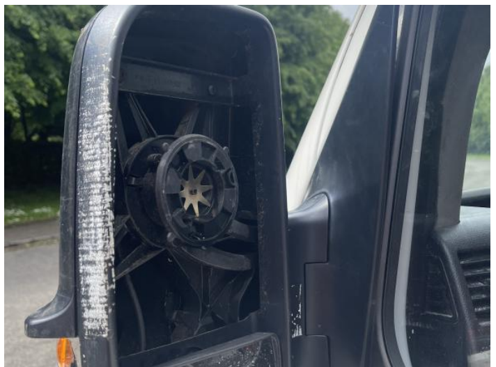
14: Door Mirror Glass ns Missing Replace
