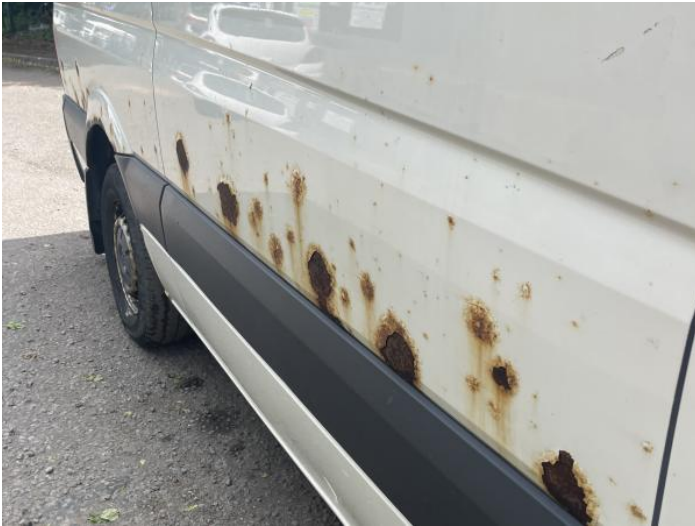
9: Qtr Panel osr Rusted Over 5mm
