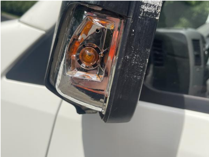
15: Door Mirror Glass ns Missing Replace
