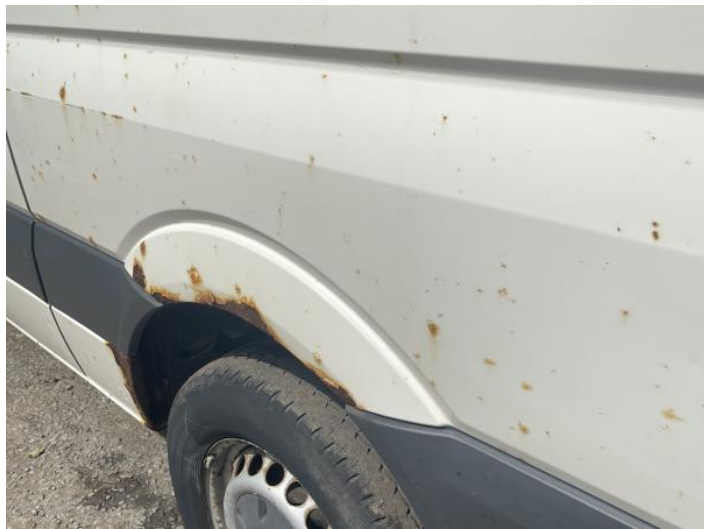
12: Qtr Panel nsr Rusted Over 5mm
