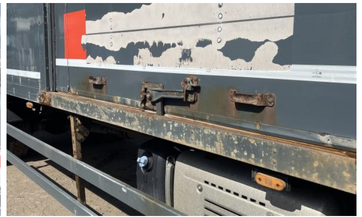
4: Bumper Front Rusted Over 5mm
