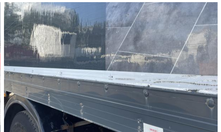
6: Qtr Panel osr Rusted Over 5mm
