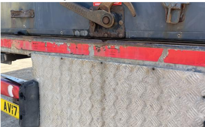
5: Door osf Dented With Paint Damage
