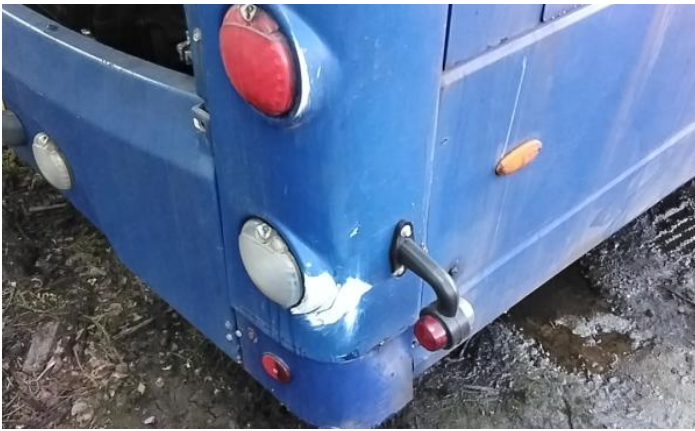
9: Qtr Panel nsr Dented With Paint Damage
