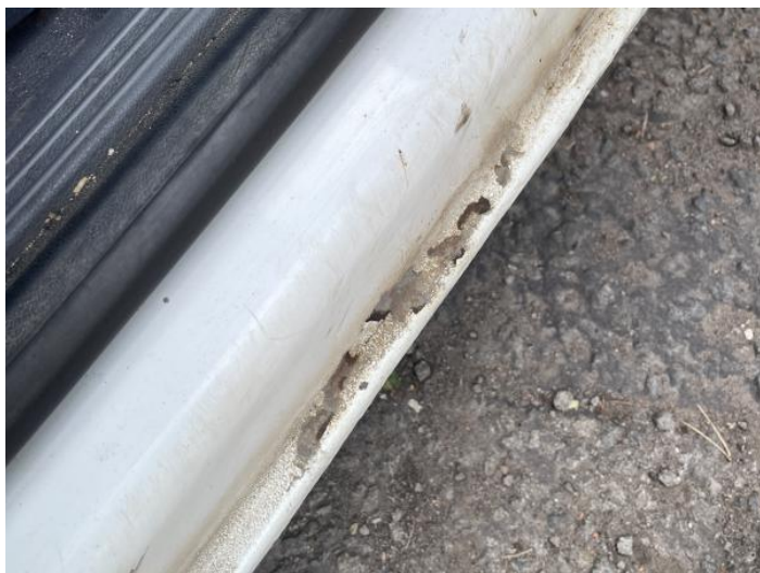
1: Sill os Rusted Over 5mm
