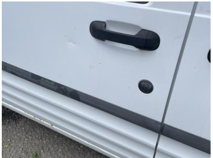
10: Door nsf Dented Over 30mm
