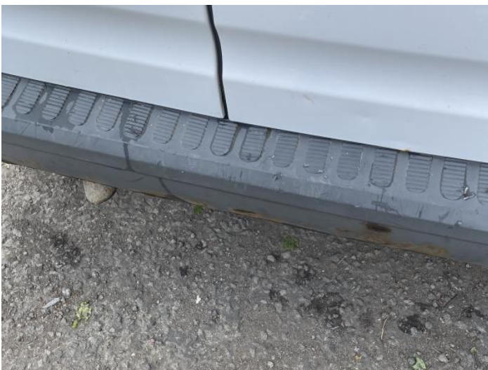
7: Bumper Rear Moulding Scuffed (Unpainted) Over 100mm
