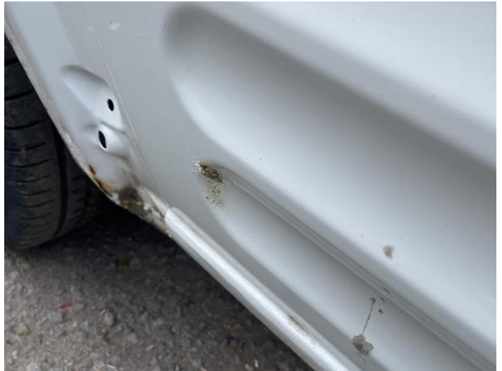
4: Qtr Panel osr Rusted Over 5mm
