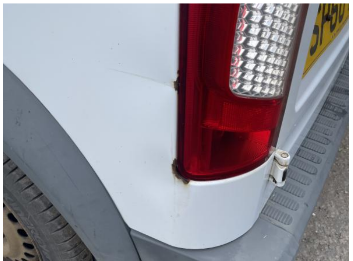
8: Qtr Panel nsr Rusted Over 5mm
