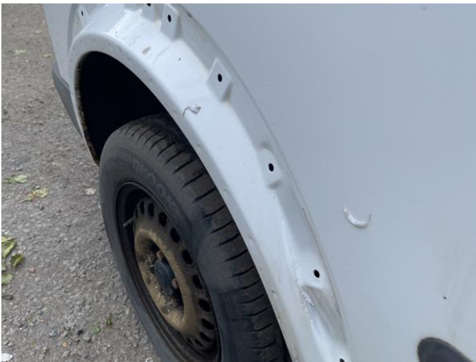
5: Qtr Panel Moulding os Missing Replace
