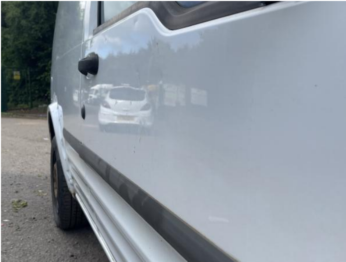
3: Door osf Dented Over 30mm
