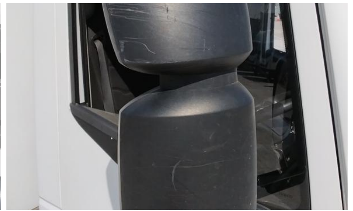
10: Moulding nsf Wing Scuffed (Unpainted) UpTo 100mm
