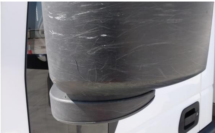
5: Moulding nsf Wing Scratched (Painted) Over 25mm Thru Paint
