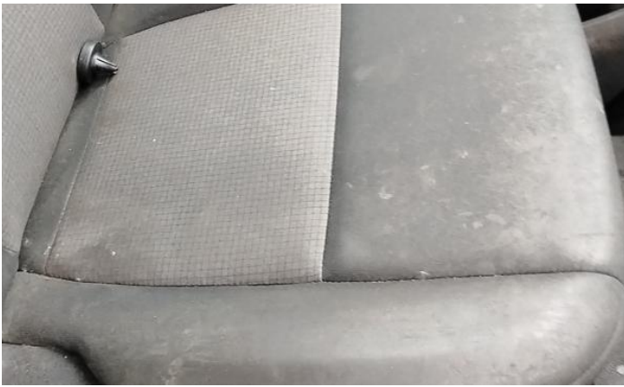
21: Seat Base Cover osf Holed Over 3mm
