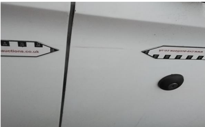
15: Qtr Panel osr Dented Over 30mm
