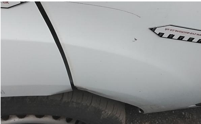
5: Wing nsf Dented Over 30mm
