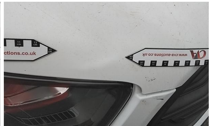
16: Qtr Panel osr Dented Over 30mm
