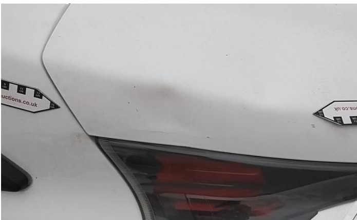
17: Door osf Scratched Over 25mm Not Thru Paint
