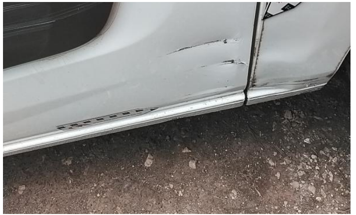
10: Qtr Panel Moulding ns Scratched (Painted) Over 25mm Thru Paint
