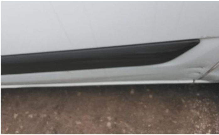
9: Door nsf Dented With Paint Damage
