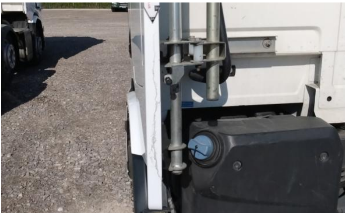
5: Wing Front Arch Extension ns Broken Replace
