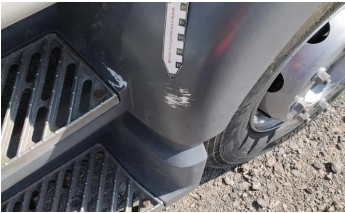
3: Bumper Front Scratched Over 100mm Thru Paint
