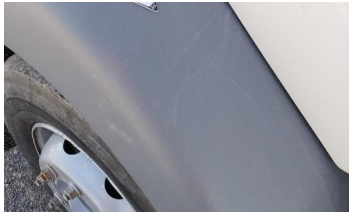
4: Door nsf Scratched Over 25mm Thru Paint
