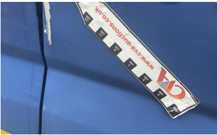
3: Bonnet Dented Over 30mm
