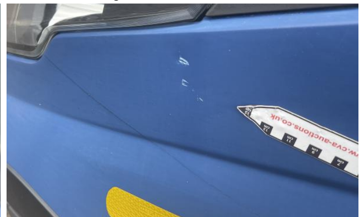
12: Door nsf Dented With Paint Damage
