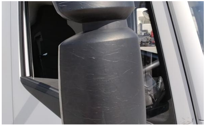
4: Door Mirror Assy nsf Scuffed (Unpainted) Over 100mm
