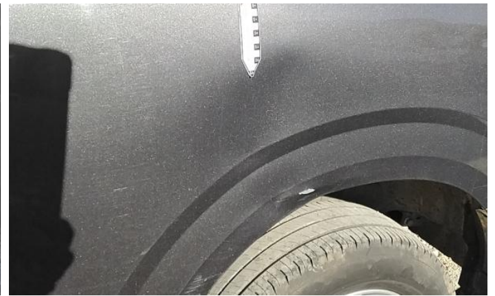
6: Door nsr Dented With Paint Damage
