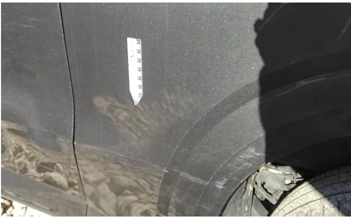
5: Door nsf Scratched Over 25mm Thru Paint
