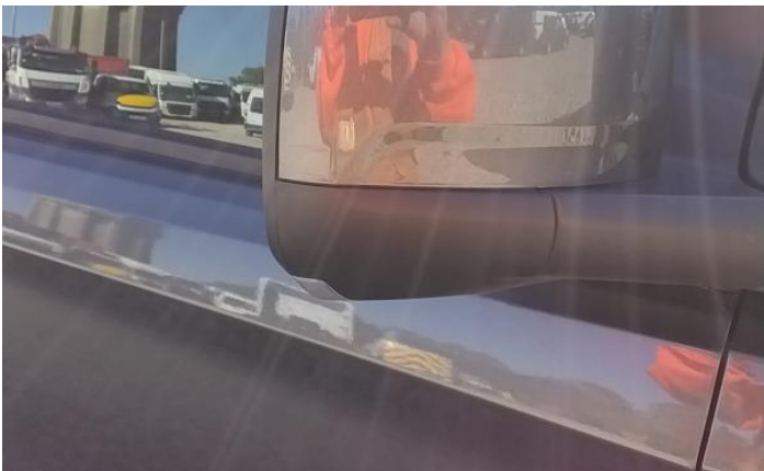
11: Door nsr Dented With Paint Damage
