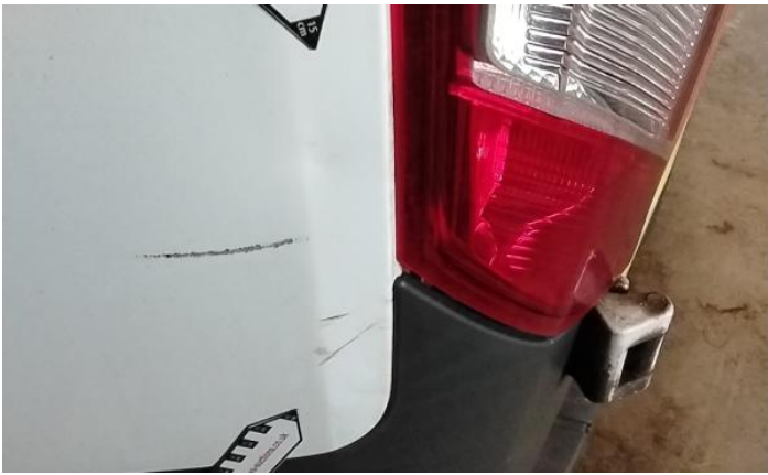
3: Qtr Panel nsr Dented With Paint Damage
