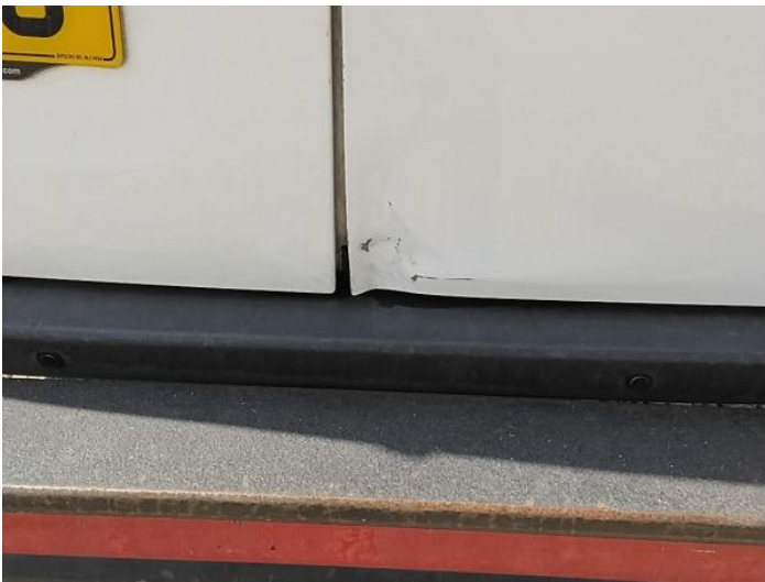
17: Door osr Dented With Paint Damage
