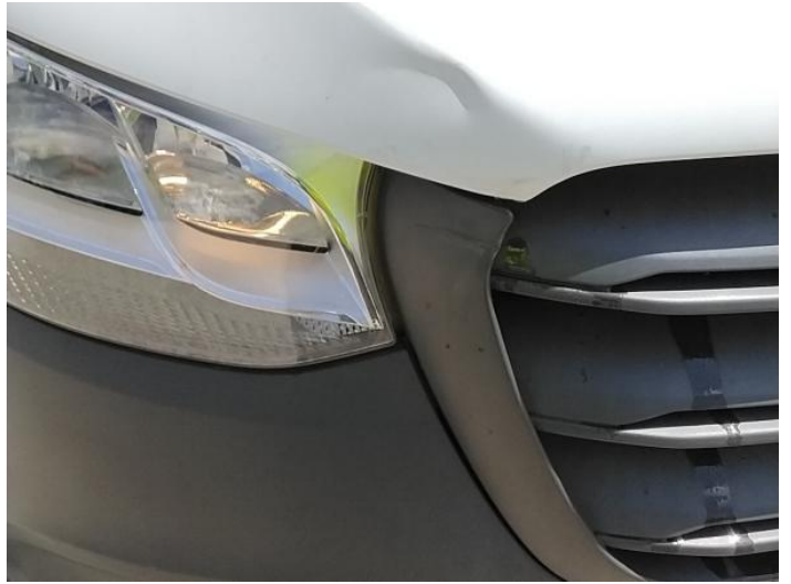
4: Bonnet Dented Over 30mm
