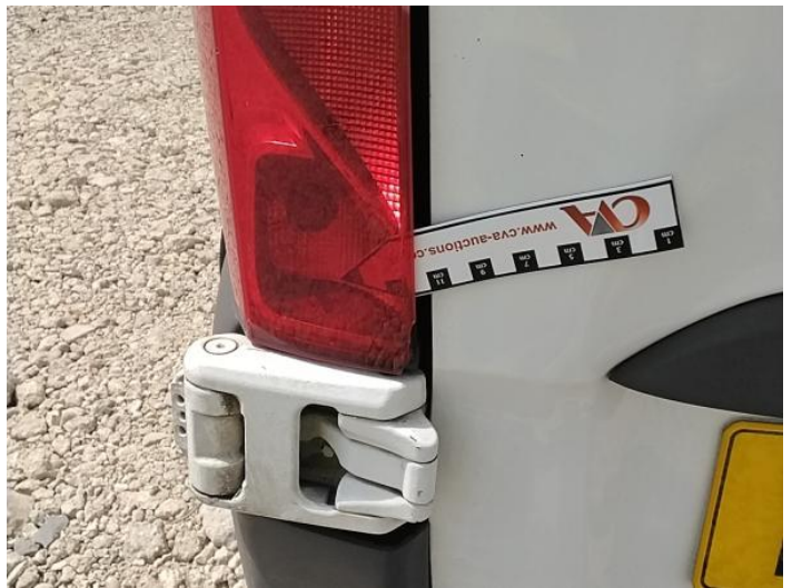
18: Lamp nsr Broken Replace
