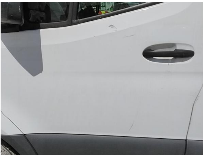
7: Door nsf Scratched Over 25mm Thru Paint
