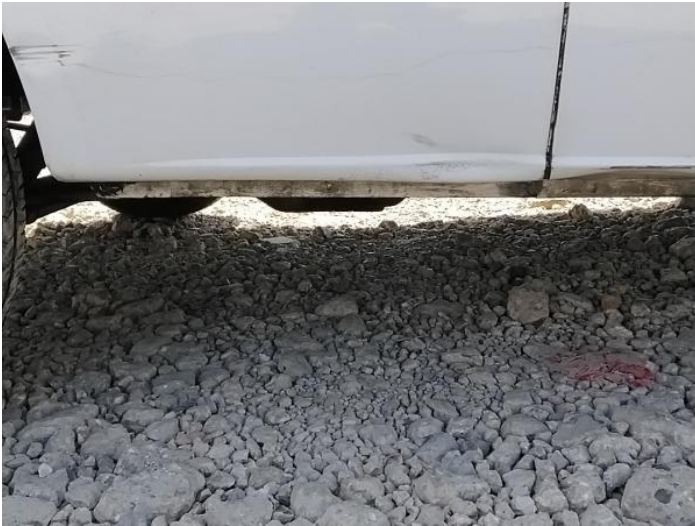
21: Sill os Dented With Paint Damage
