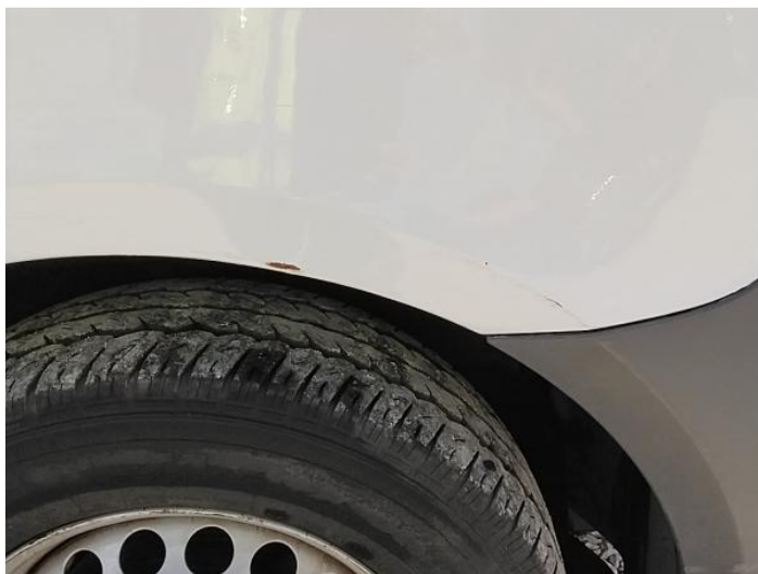
1: Wing osf Rusted Over 5mm
