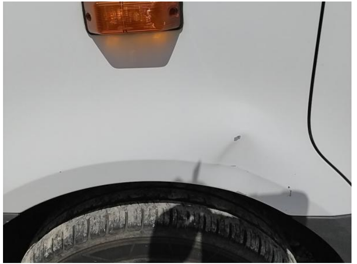
6: Wing nsf Dented With Paint Damage
