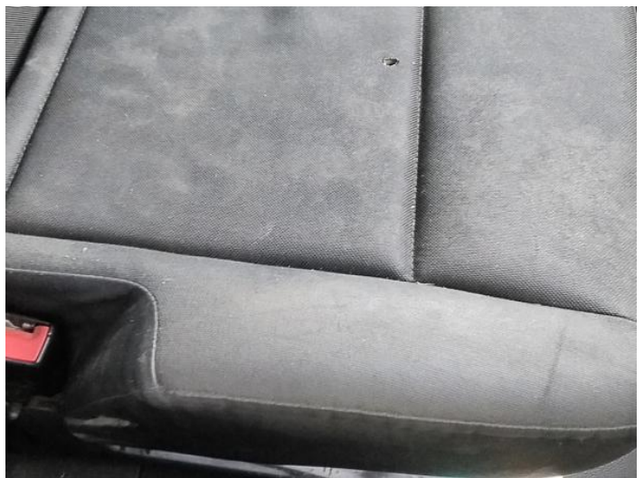
26: Seat Base Cover nsf Holed Over 3mm
