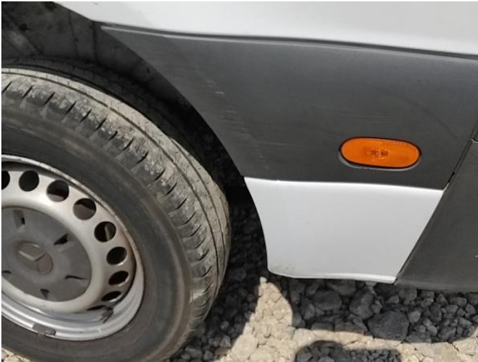
15: Qtr Panel nsr Scratched Over 25mm Not Thru Paint
