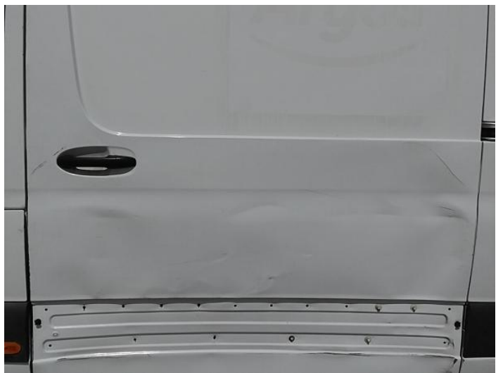
8: Door nsr Dented Over 30% Of Panel
