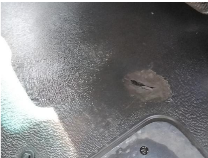
25: Carpets Front Holed Over 3mm
