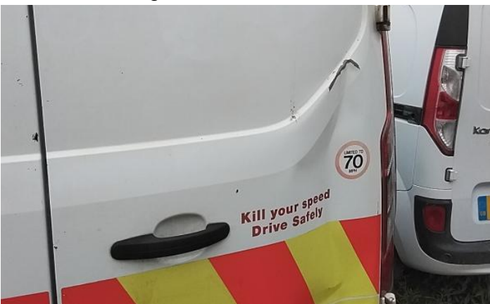
5: Qtr Panel nsr Dented With Paint Damage
