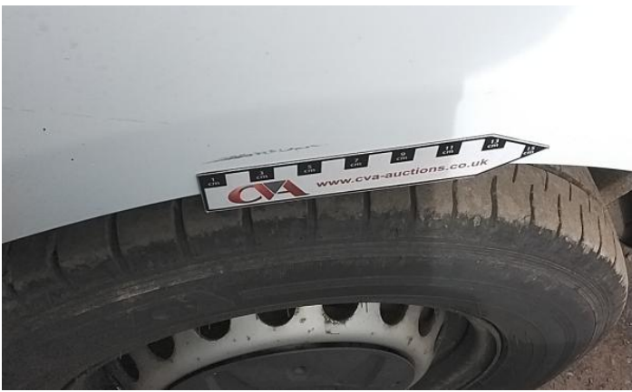
9: Qtr Panel osr Dented With Paint Damage
