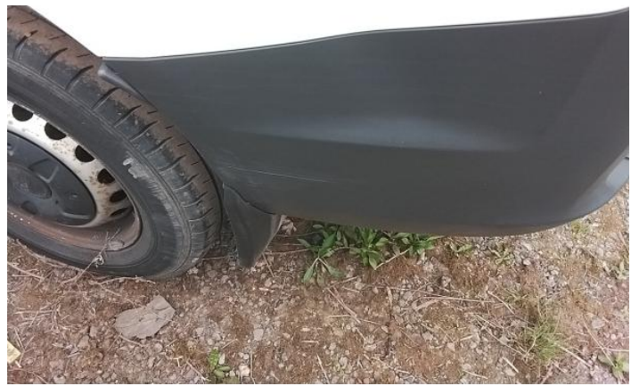
4: Qtr Panel nsr Dented Over 30mm
