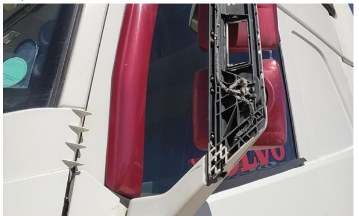
6: Wing nsf Cracked Replace
