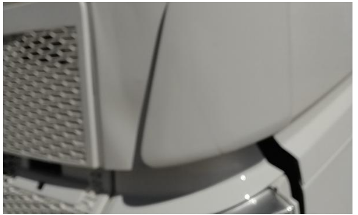
4: Screen Front Chipped Up To 10mm
