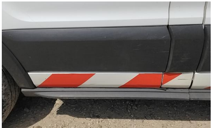
6: Door nsf Scratched Over 25mm Not Thru Paint
