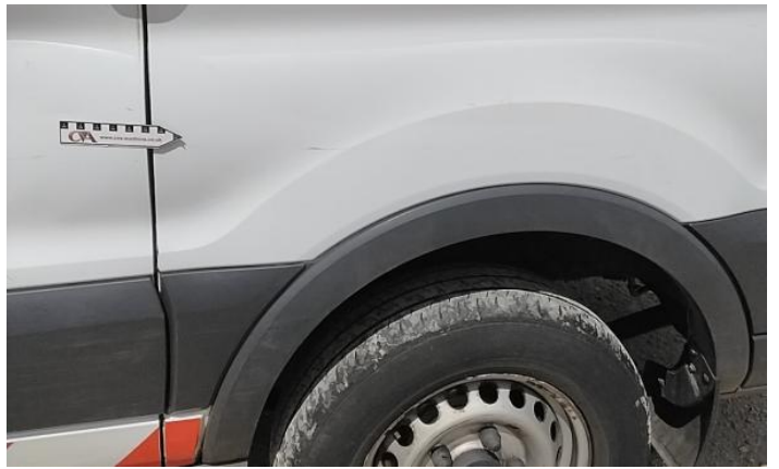
10: Door nsr Dented Over 30% Of Panel
