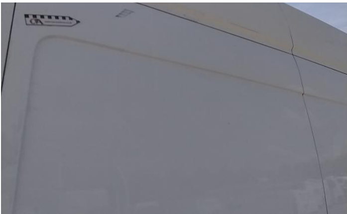
11: Door nsr Dented Between 10mm + 30mm
