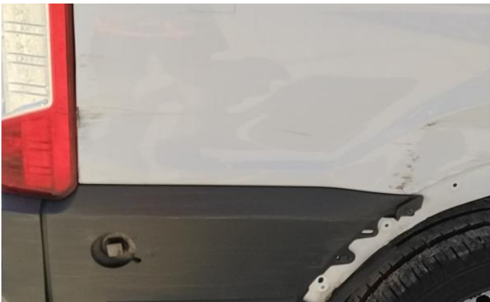
17: Bumper Rear Dented Over 30mm
