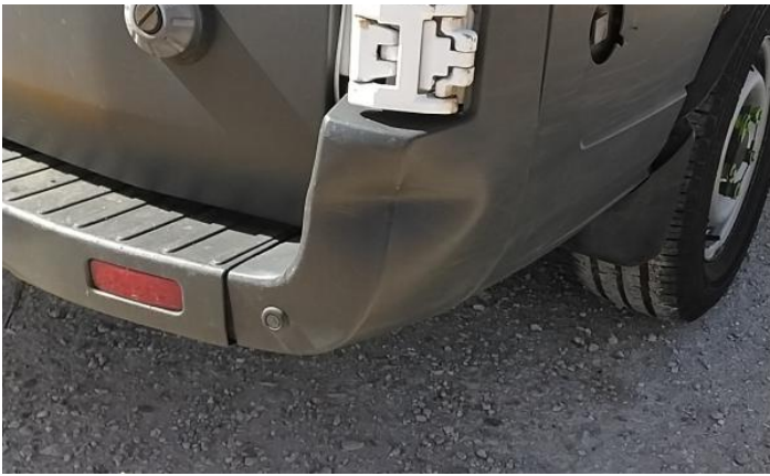
15: Bumper Rear Moulding Scuffed (Unpainted) Over 100mm
