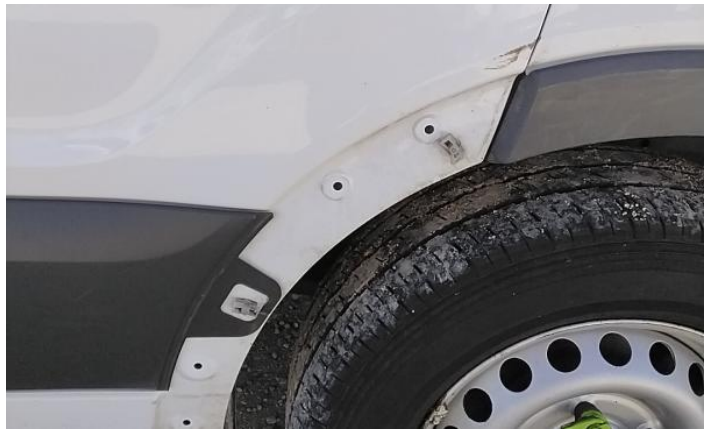
22: Qtr Panel osr Dented With Paint Damage
