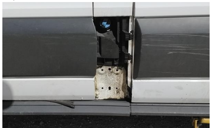
6: Flasher Side Repeater ns Broken Replace
