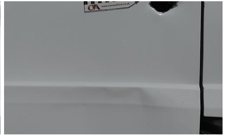
10: Door Moulding nsr Scuffed (Unpainted) Over 100mm
