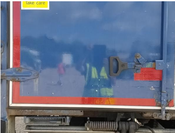
11: Door nsr Scratched Over 25mm Thru Paint
