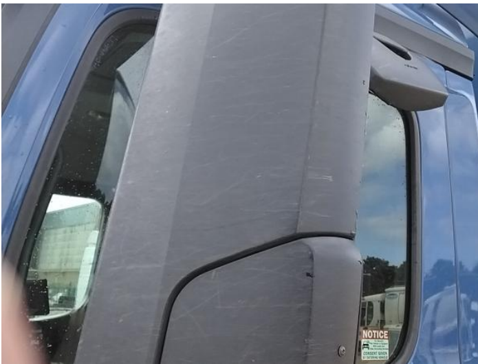
5: Door Mirror Assy nsf Broken Replace
