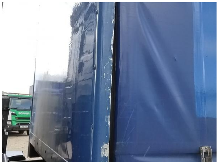
8: C Post ns Scratched Over 25mm Thru Paint
