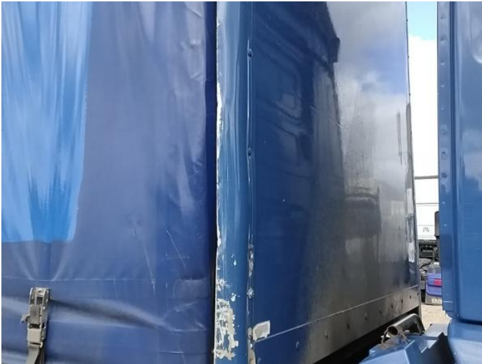
15: C Post os Scratched Over 25mm Thru Paint
