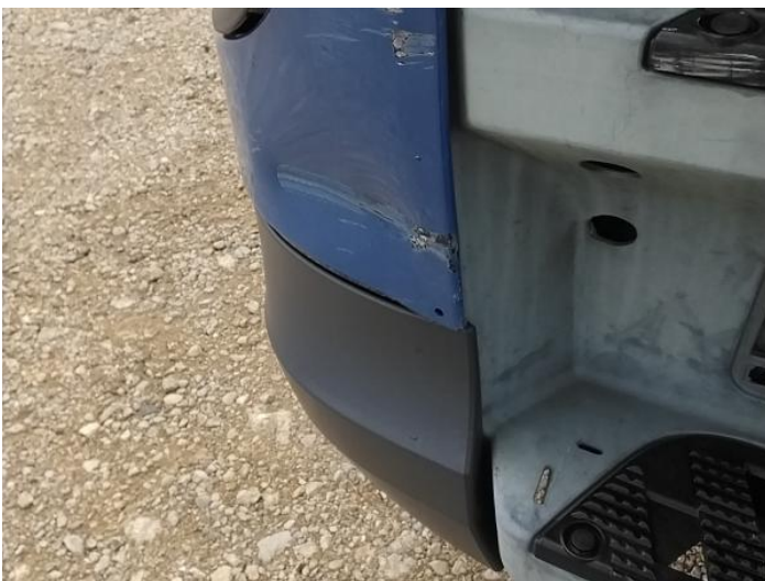
7: Moulding nsf Wing Scratched (Painted) Over 25mm Thru Paint
