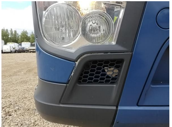
2: Moulding of Wing Scratched (Painted) Over 25mm Thru Paint
