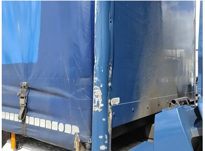
16: C Post os Dented With Paint Damage
