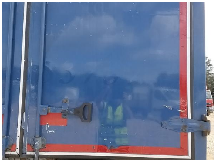
12: Door osr Scratched Over 25mm Thru Paint
