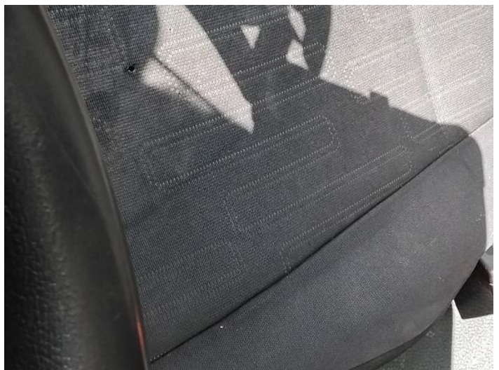
20: Seat Base Cover osf Holed Over 3mm
