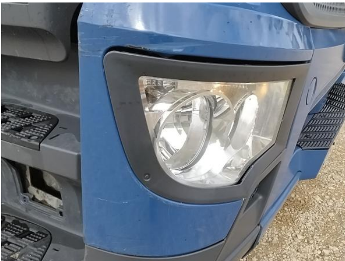
1: Moulding of Wing Scratched (Painted) Over 25mm Thru Paint
