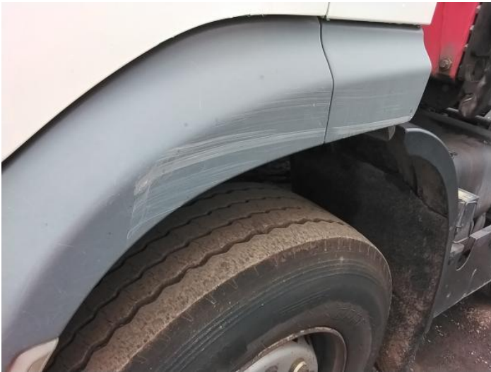
5: Wing nsf Scratched Over 25mm Thru Paint
