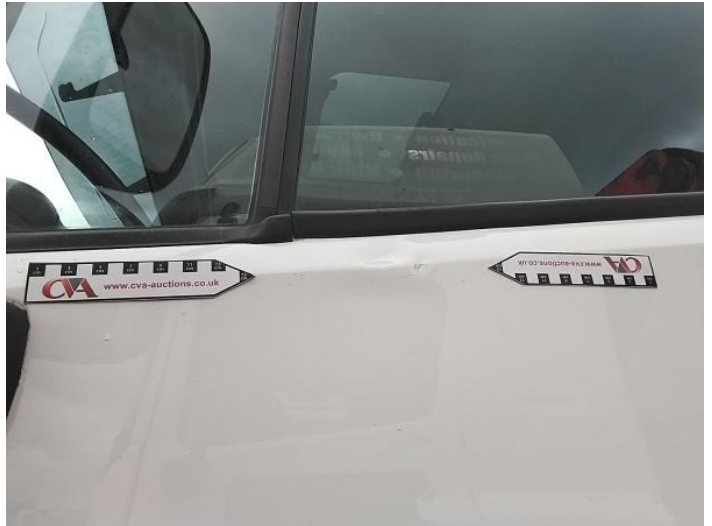
4: Door nsf Dented Over 30mm
