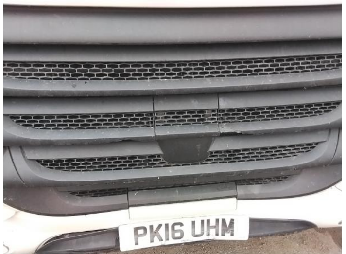
2: Bumper Front Grill Broken Replace
