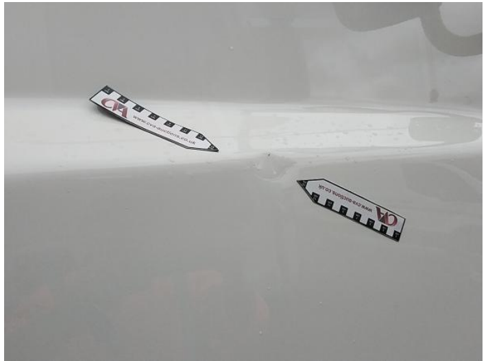
6: Door osf Dented Over 30mm
