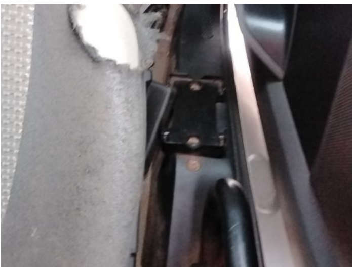
7: Seat Base Cover osf Torn Over 3mm
