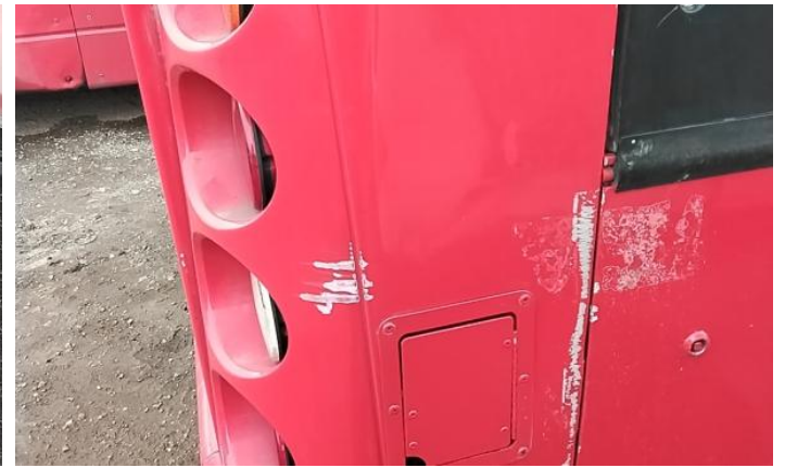
10: Bumper Rear Cracked Over 25mm
