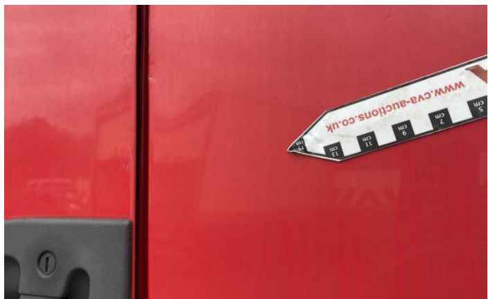
6: Qtr Panel of Rusted Over 5mm
