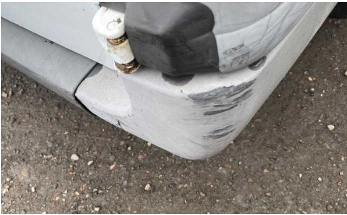
9: B Post os Rusted Over 5mm
