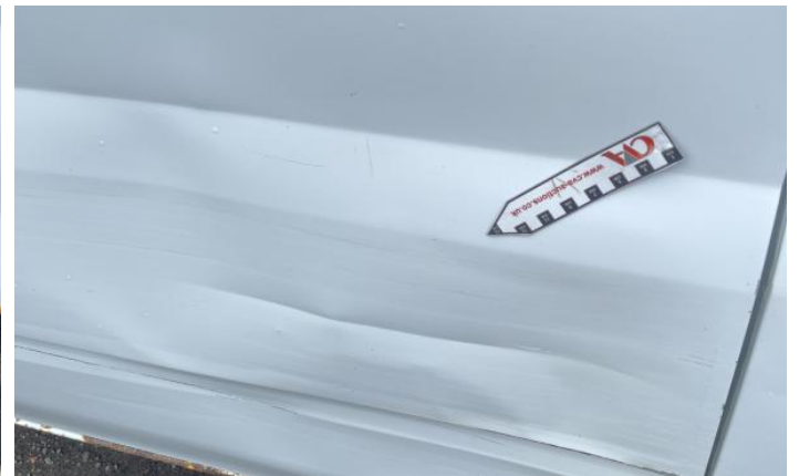
12: Tailgate Dented With Paint Damage
