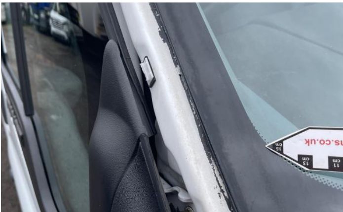
5: Wing of Rusted Over 5mm
