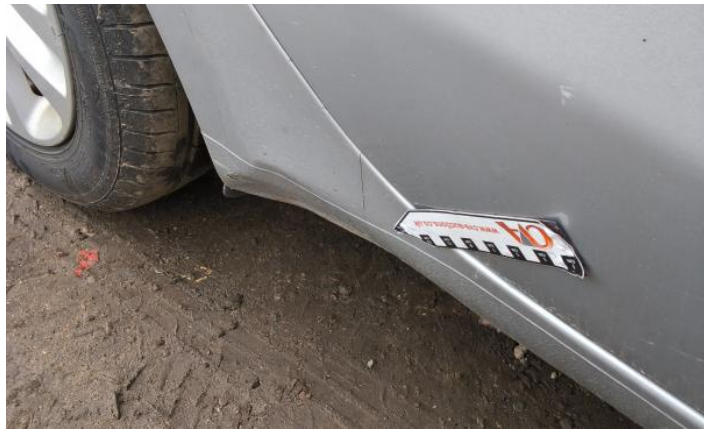
4: Bumper Front Cracked Over 25mm
