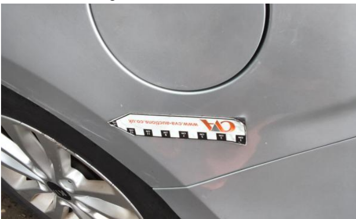
5: Wing osf Dented With Paint Damage
