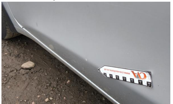
6: Sill os Dented With Paint Damage
