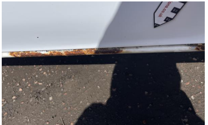
6: Qtr Panel osr Dented With Paint Damage
