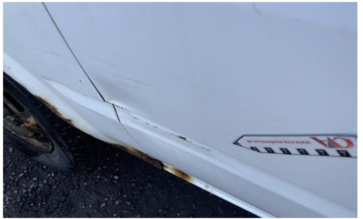
4: Door osf Rusted Over 5mm
