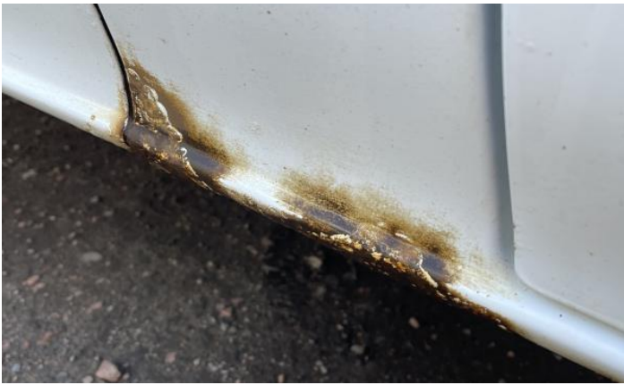
3: Wing osf Rusted Over 5mm
